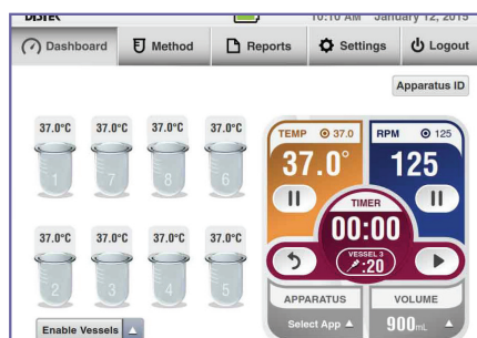
Dashboard screen with wireless in-shaft temperature sensors
